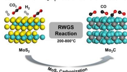
Figure.1. Dynamic transformation of MoS<sub>2</sub> catalysts to Mo<sub>2</sub>C phase under RWGS reaction
